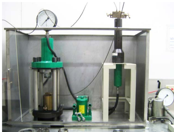
Fig. 2. Pressure intensifier and device for hydrogen pressures up to 15 kbar.
